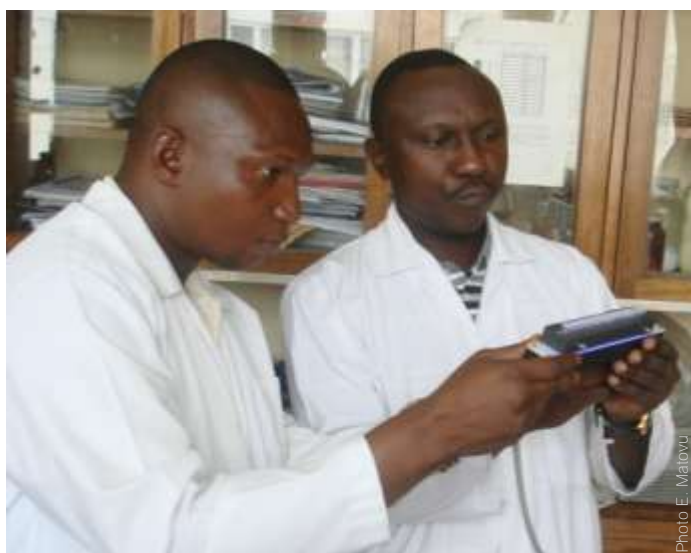
Reading LAMP results with an LED light source.
